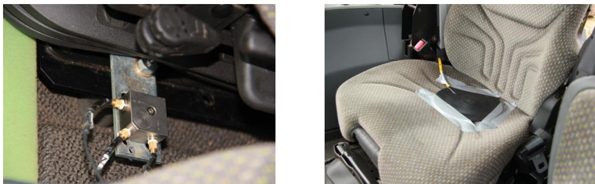
Figure 2: illustration of the mounting of the accelerometers at the chair base (left) and on the seat (right).
