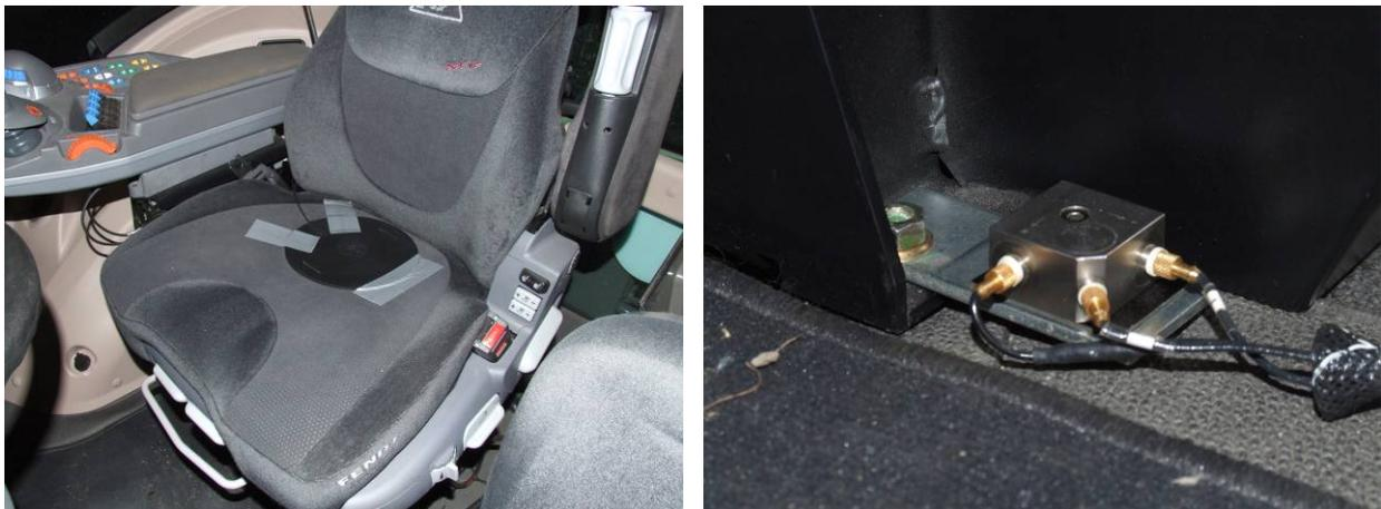
Figure 2: illustration of the mounting of the accelerometers on the seat (left) and at the chair base (right).
