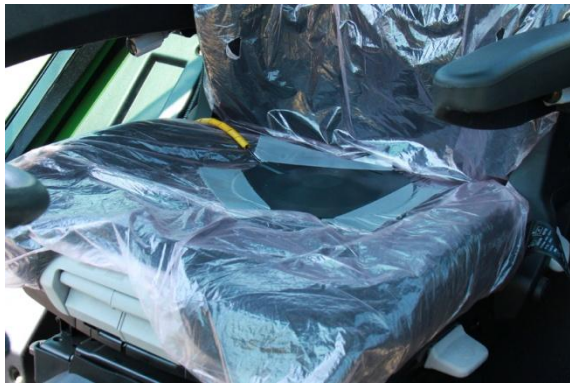
Figure 3: Illustration of the of the mounting of the accelerometer pad on the seat.
