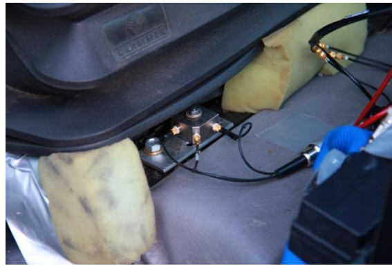
Figure 4: Illustration of the of the mounting of the accelerometer at the chair base.
