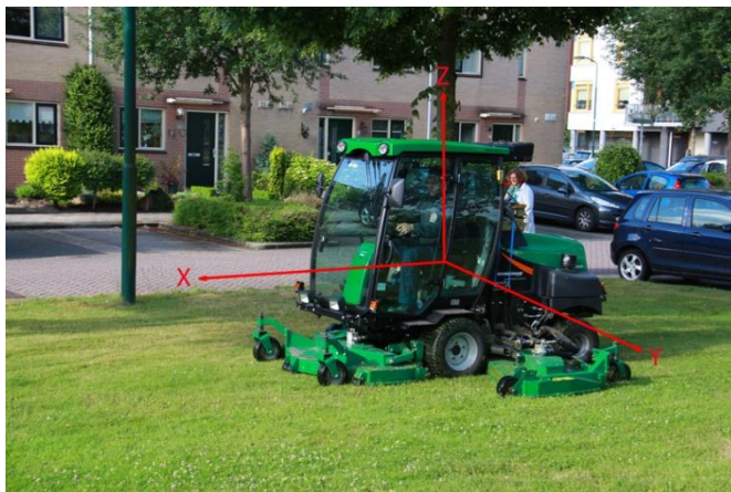
Figure 2: Visual illustration of the vibration axes X, Y and Z.
