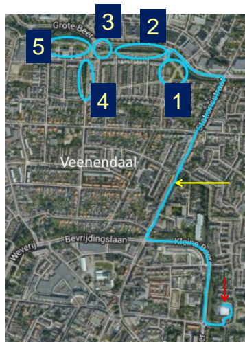
Figure 1: View on the measurement location. On the map (obtained via Google Maps) are indicated the starting location (red arrow), route for driving to and from the plots (yellow arrow) and the five testing plots of public green area. Plots 1+2: normal speed; plots 3+4: hasty speed; plot 5: restrained speed.
